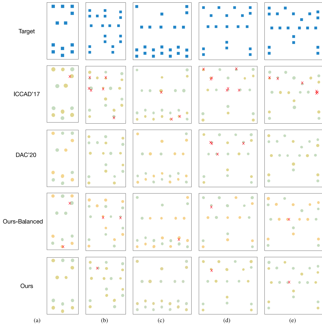
Fig. 12. Comparison with ICCAD'17 [9] and DAC'20 [28] on: (a) BUF_X1; (b) OAI211_X1; (c) NAND3_X2. (d) NOR3_X2. (e) OAI33_X1. Compared with the state of the art, in all five cases, our framework results in fewer EPEs.
