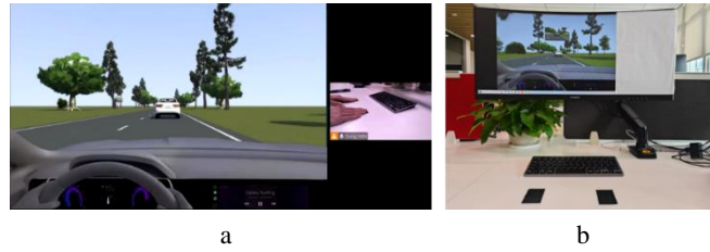
Figure 1: The setup for the video simulation experiment: a) screenshot of the driving scenario and the place of participants' hands; b) the apparatus for the experiment.
