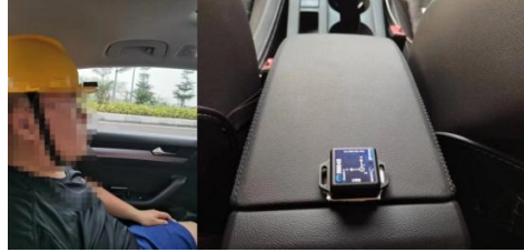
Figure 2: The positions of the IMUs for recording the head poses and vehicle dynamic profile.
