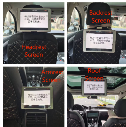
Figure 1: The four different display positions investigated in the study.
