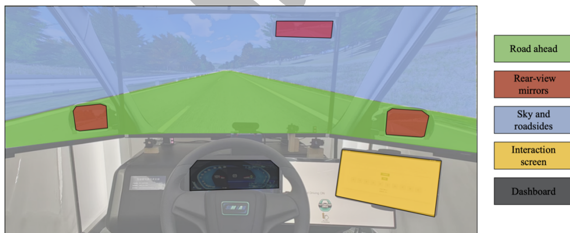
Figure 7. Five areas of interest (AOIs) for eye-tracking analysis: road ahead, rear-view mirrors, sky/roadsides, NDRT interaction screen, and dashboard.
