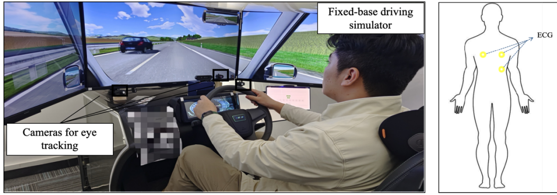
Figure 1. Driving simulator, eye-tracker, and physiological sensor placements.
