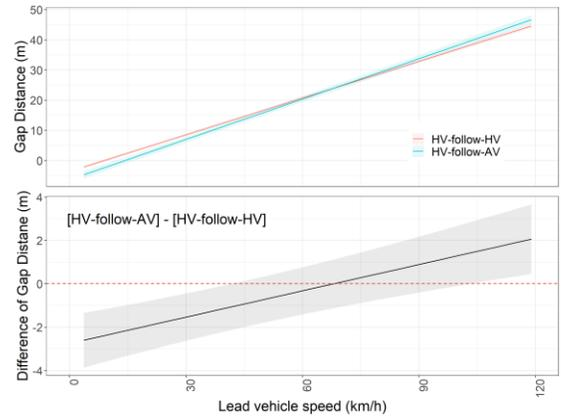
Figure 2. The results of the gap distance model. In this figure and the following figures, the shadow represents 95% confidence interval (CI) of the estimated differences between the two types of car-following events.
