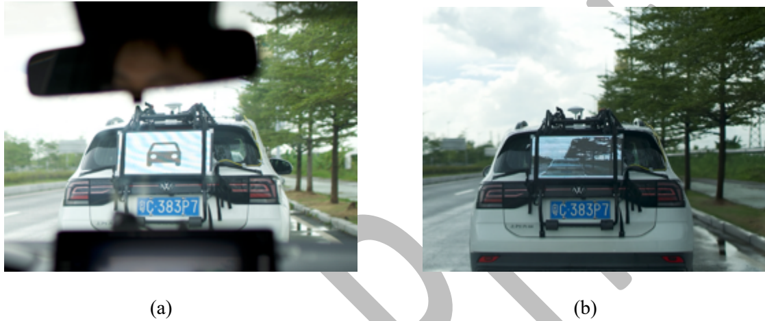
Figure 3 The eHMIs used in the experiment (a) Brake-eHMI; (b) Video-eHMI.
